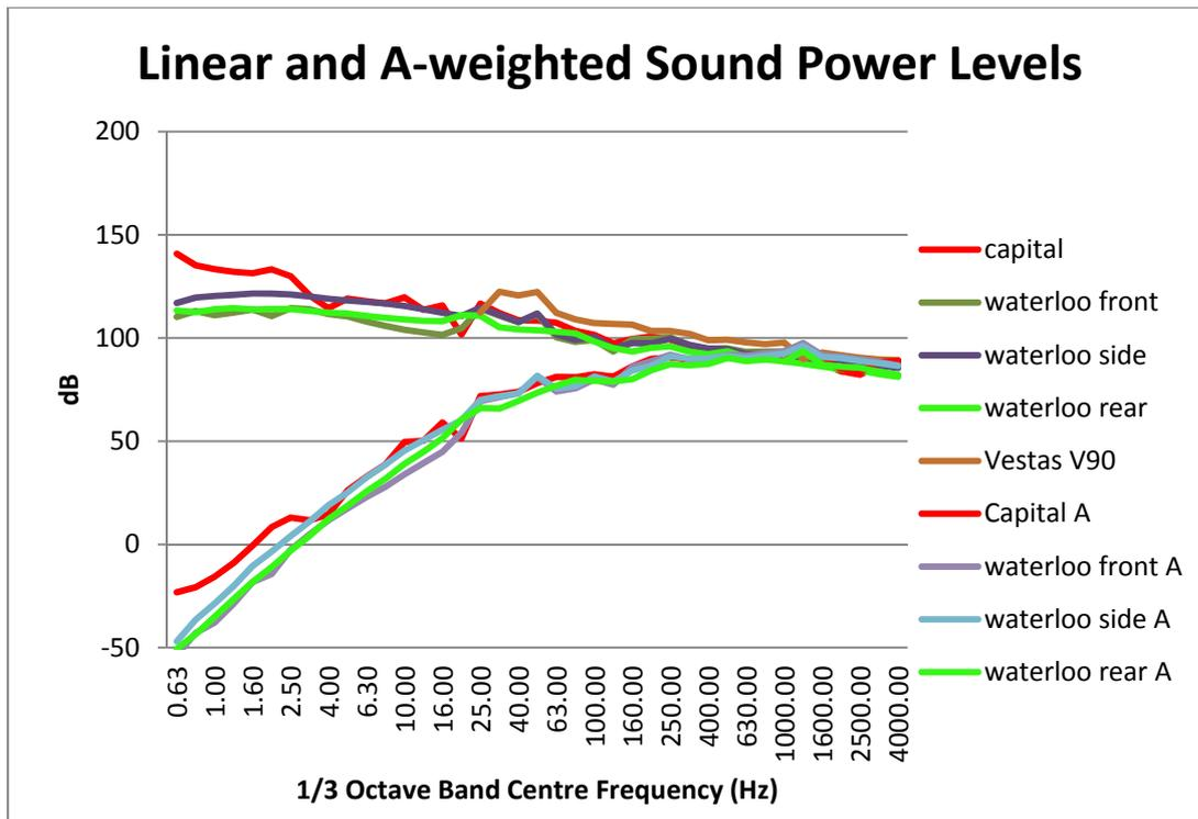
**FIGURE 3 Turbine Sound Power Levels (Linear versus A-weighted)**
