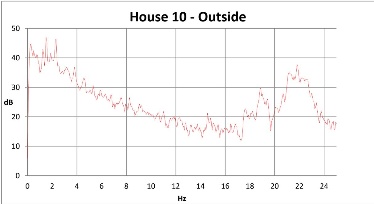
**FIGURE 8 External Measurements approximately 1300 metres from nearest turbine**
