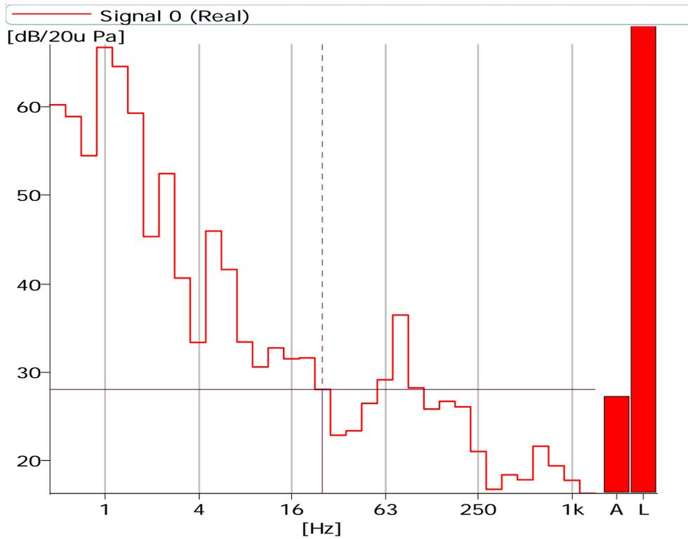
**FIGURE 10 External Measurements approximately 8000 metres from nearest turbine**
