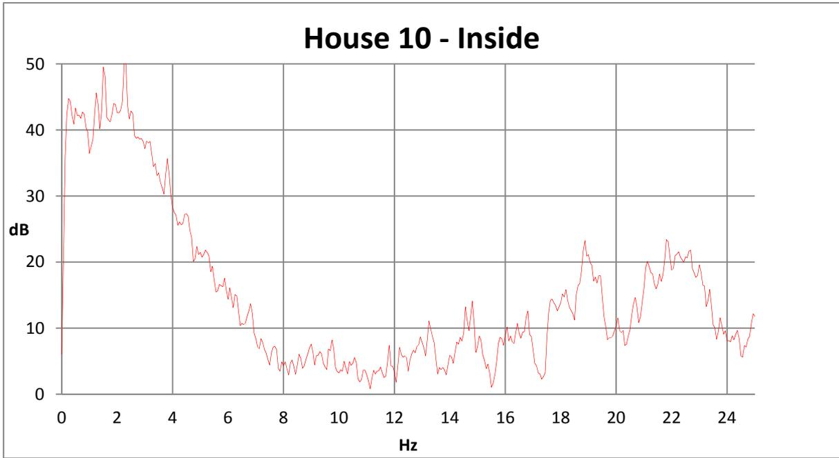
**FIGURE 9 Internal Measurements approximately 1300 metres from nearest turbine**
