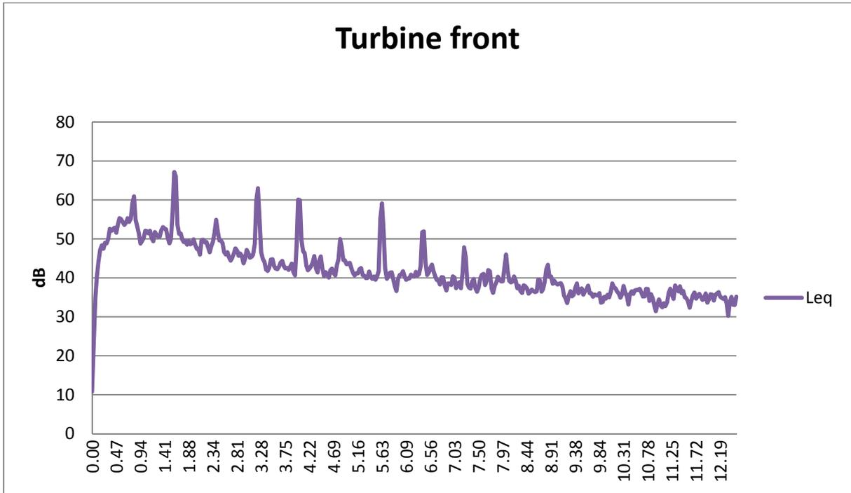
**FIGURE 7: 0 – 12.5 Hz at 150 metres from tower**
