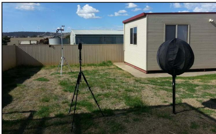
**Figure 1 – Picture of the EPA microphones and weather station at the “township” site.**
